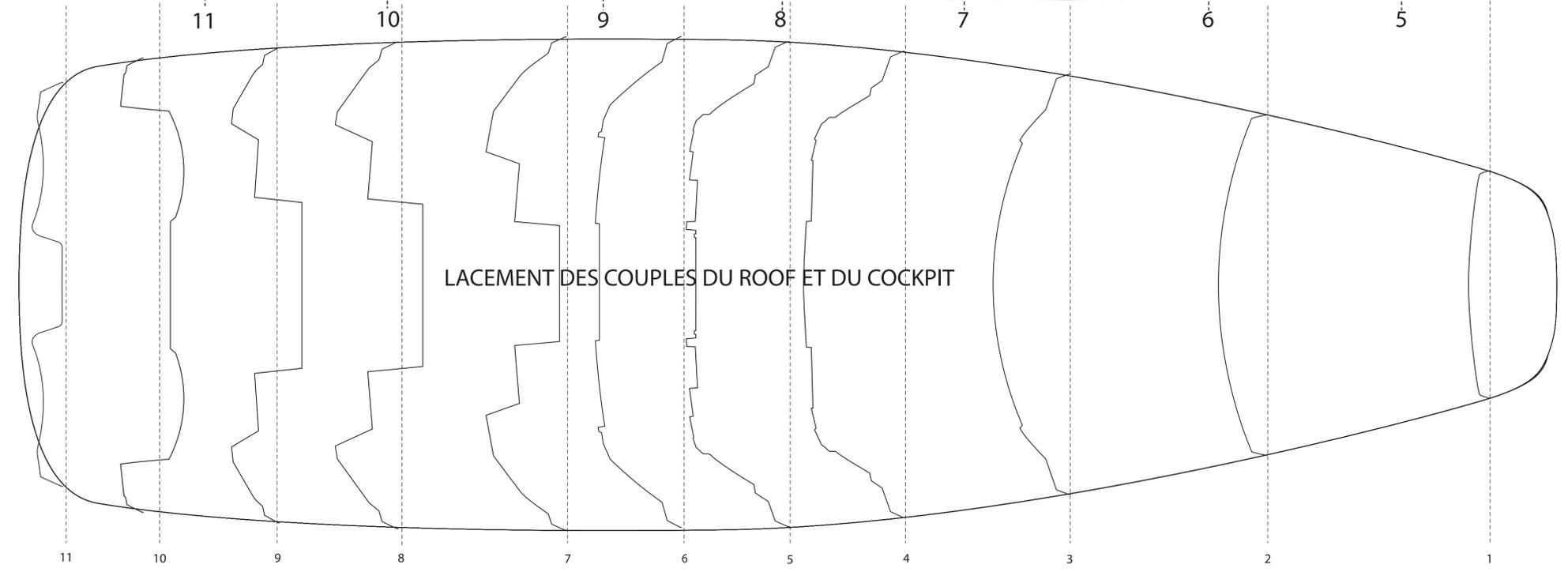
LACEMENT DES COUPLES DU ROOF ET DU COCKPIT
